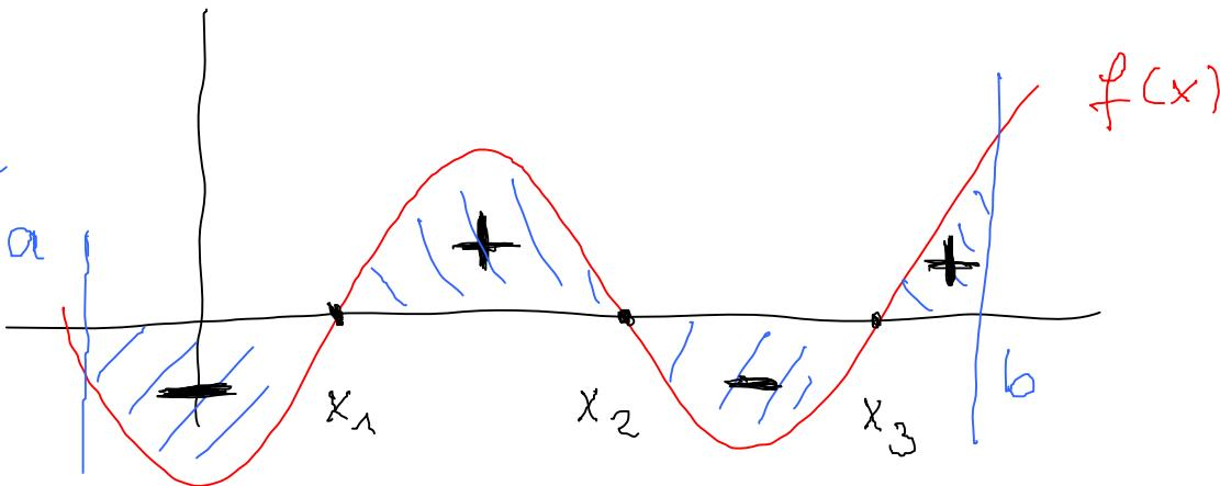
$$A = \int_a^b f(x) dx = \left| \int_a^{x_1} f(x) dx \right| + \left| \int_{x_1}^{x_2} f(x) dx \right| + \left| \int_{x_2}^{x_3} f(x) dx \right| + \left| \int_{x_3}^b f(x) dx \right|$$
