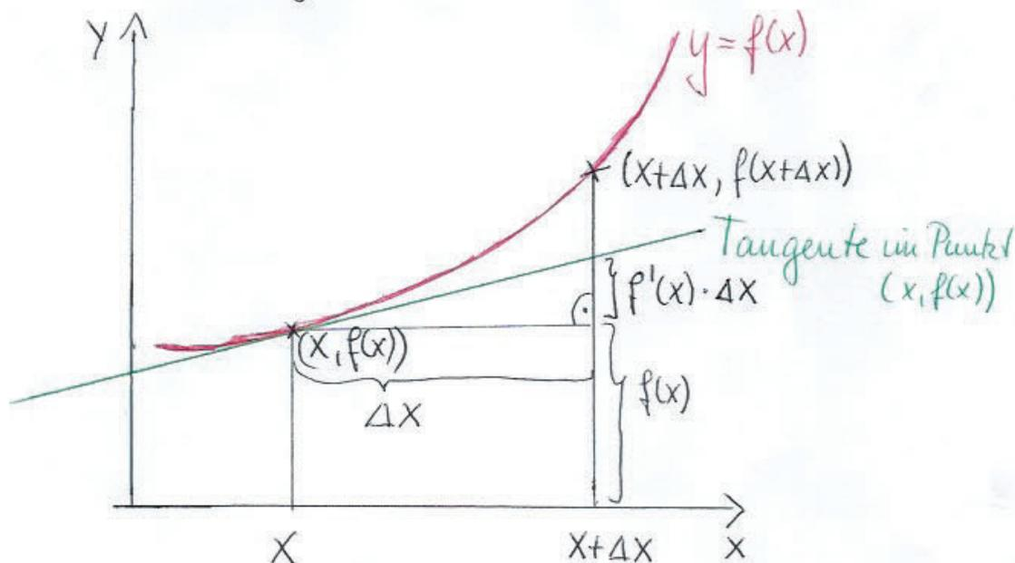
$$f'(x) = y' = \frac{dy}{dx} \text{ Differentialquotient}$$
