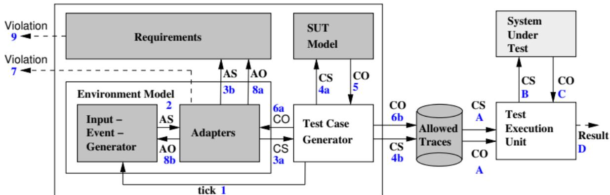
The test case generator simulates the SUT in its environment and stores the resulting test cases.
