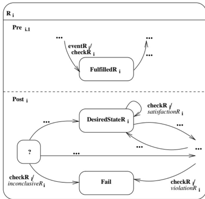
The **postcondition** of the requirement is checked when all **preconditions** are fulfilled.
