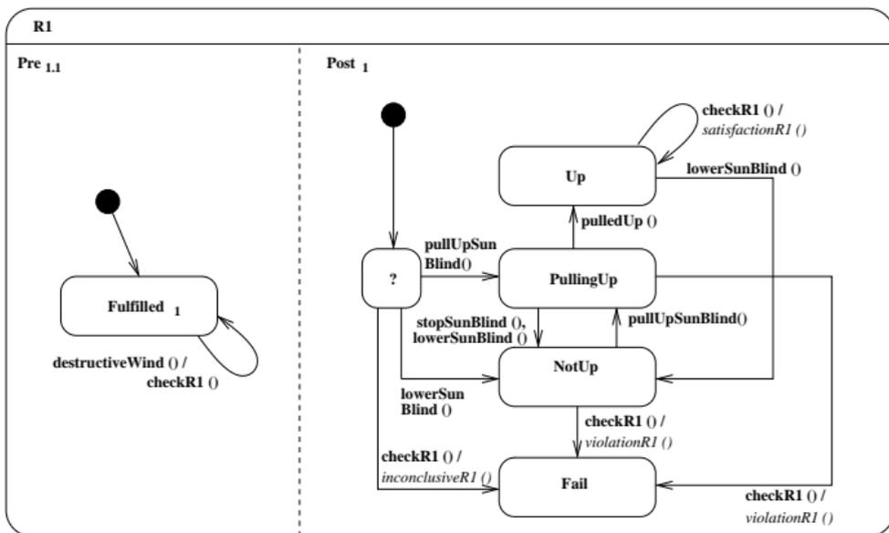
If there is destructive wind, it must be checked if the sunblind is up. If yes, the requirement is satisfied. Otherwise, it is violated. The *Fail* state corresponds to a state where the sunblind would be destroyed.
